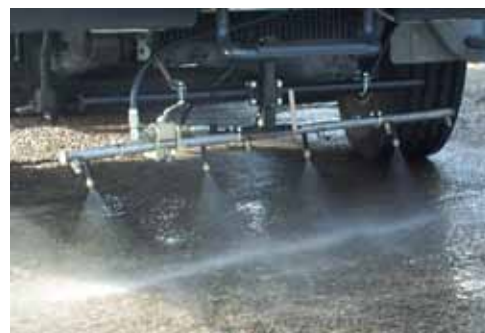
Figure 5b. High Pressure Spray bar on front bumper
