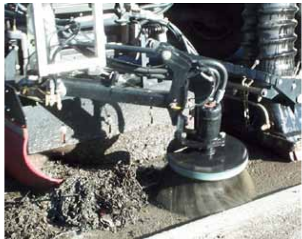
Figure 1. Side-mounted channel brush with suction nozzle
